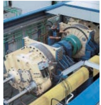
Rexroth gearbox under full-load test in test bench
