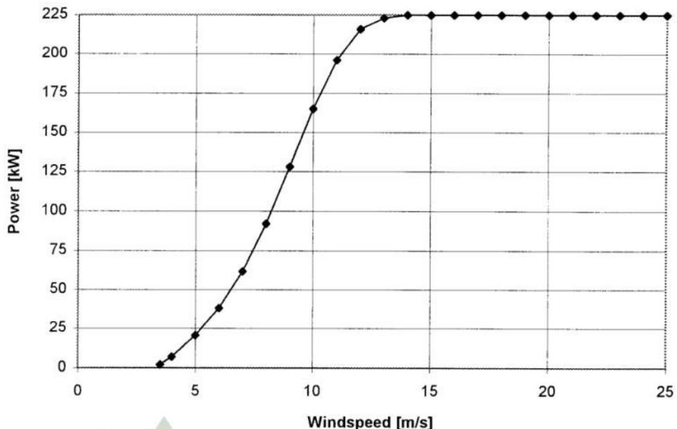
The V29-225 kW power curve is based on measurements performed by WindTest, Tripod and Vestas. The power curve is calculated with a mean density of  $1.225 \text{ kg/m}^3$  and a turbulence of 10 %. The curve will vary at other values of turbulence and air density.
