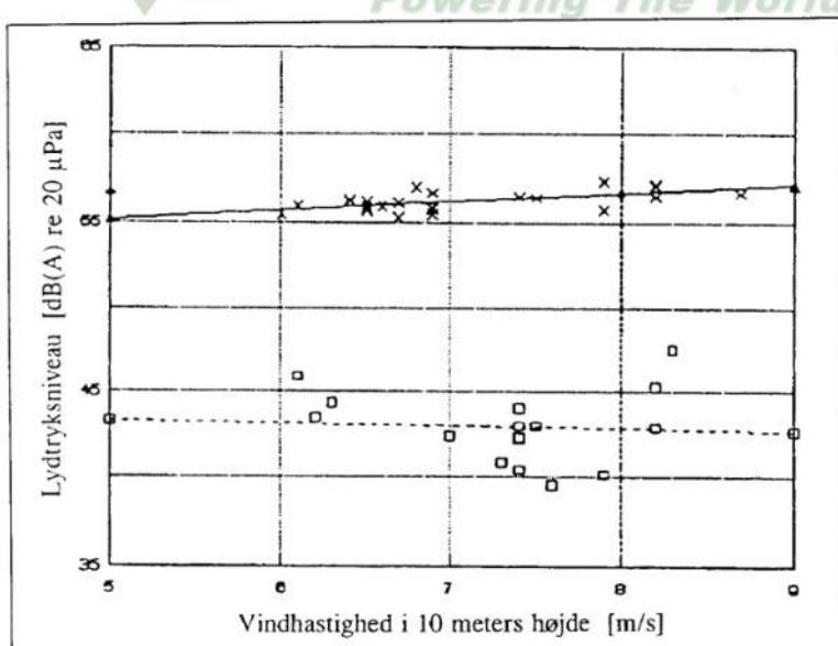
The sound power level ( $L_{Aeq}$ ) can be calculated from the sound pressure level, using the following expression:
